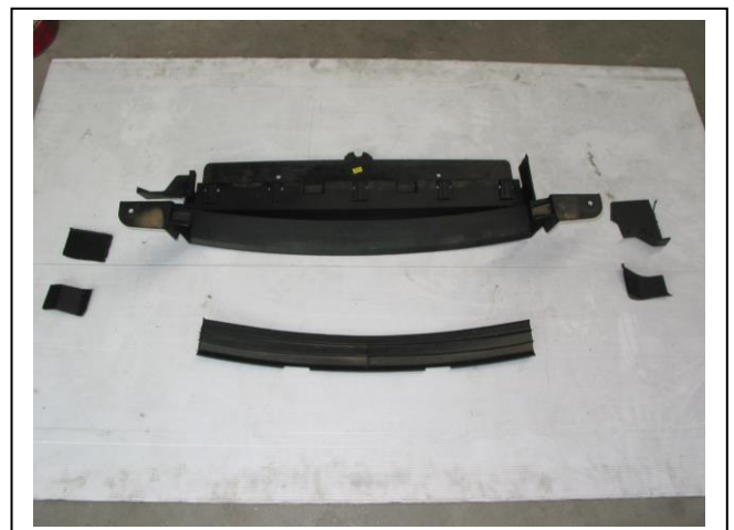
Figure 18 – Adventra and Cross 8 shown Air dam trimmed to fit around steel mounting brackets
